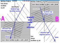
Wave fronts makes it easier to visualise loads of waves moving together. If we show movement of light from air into glass, when the first wave fronts start to move into glass, they slow down; they move closer together and the wavelength decreases. So, the speed slows down because the frequency stays the same. The amount of infrared radiation absorbed or radiated by a surface depends on the nature of that surface, e.g. colour.
