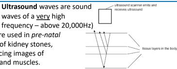
Ultrasonic waves are partially reflected when they meet a boundary between different materials. The distance of a boundary is calculated by measuring the time taken for the wave to return to the detector and knowing the speed of sound in the medium.
